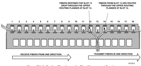
Figure 701-2. Routing Fiber Across the Fiber Management Panel
